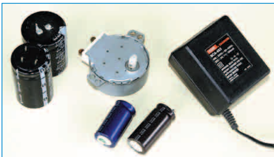
The primary components needed are the turntable motor from a microwave oven, an old plugpack and some high-value, low-voltage capacitors. These salvaged parts shouldn't total more than a few pounds, but do be careful when salvaging the turntable motor – the bite from the EHT circuitry in a microwave oven can be lethal, even with the power off (see warning in article).
