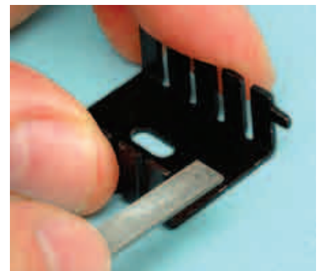
Fig.13: here's how to assemble the regulators to their heatsinks. The 7805 regulator (REG4) presents a special case; its screw should be inserted from the opposite side to that shown so that the screw head isn't obscured by REG3's heatsink.
