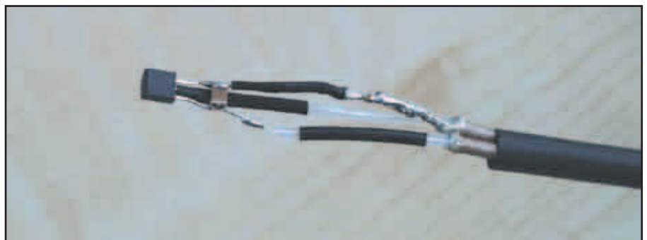
Connecting the suppression capacitor across the sensor leads
