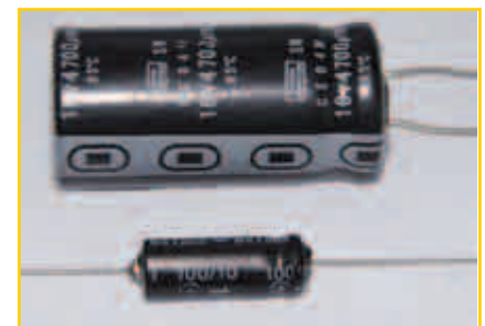
Fig.4. An axial electrolytic capacitor (bottom) has an indentation around the body at the positive end. PCM electrolytic capacitors have a similar indentation, but it is of no importance. Both types are marked with '+' and (or) '-' signs as well
