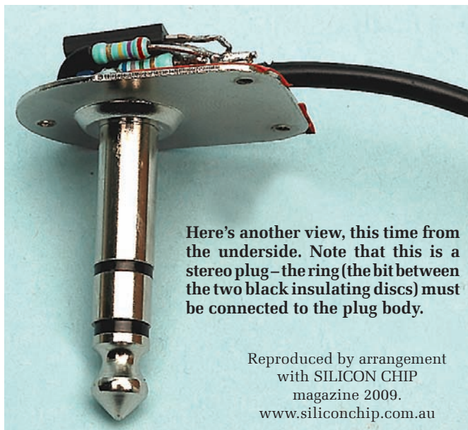
The Safe-T-Flash built onto the 6.5mm plug. We provided insulation wherever there was a risk of shorting (including the red insulation tape covering the body). The 220nF capacitor is under the SCR.
