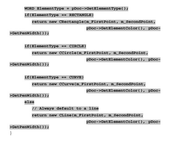
We've added a local variable ElementType to store the current element type retrieved from the document. This is then tested against the element types imported from the DLL in the series of if statements. This does exactly the same job as the switch statement, but has no requirement for the element type constants to be known explicitly. If you now build Sketcher with these changes added, it will execute using the DLL, using the exported symbols as well as the exported shape classes.
