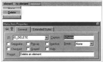
Make sure that you type sensible IDs rather than allowing the default, which is to use the junk name on the menu bar. Here, we have entered **ID\_MOVE** and **ID\_DELETE** as the IDs for the two items in the pop-up. The illustration shows the properties box for the <u>Delete</u> menu item.
