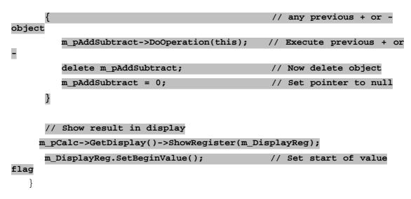
When the *Enter* key is received, all outstanding operations need to be executed and the final result displayed on the screen. The function checks the pointers m\_pMultiplyDivide and m\_pAddSubtract, performs any queued operations through the DoOperation() function, and ensures the pointers are reset to NULL.
