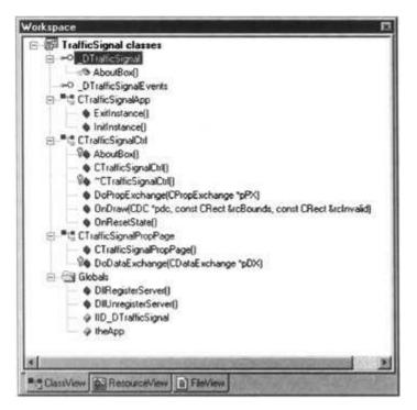
There are just three classes defined: the application class CTrafficSignalApp, the control class CTrafficSignalCtrl, and the property page class CTrafficSignalPropPage.
