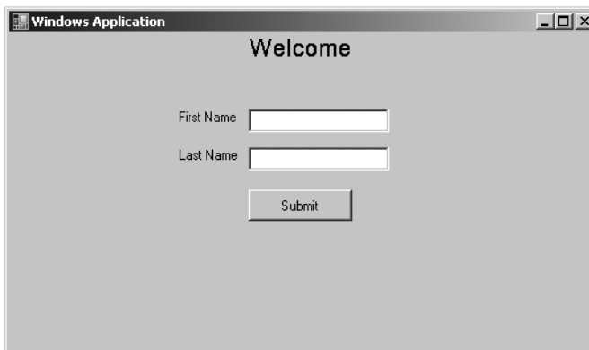
Figure 14-15. The effect of the Anchor property setting Top on a resized form
