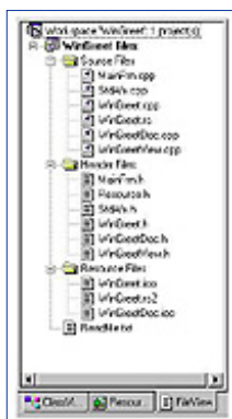
FIGURE 9.9 The graph of the WinGreet project files in the FileView tab of the Visual Studio Workspace window
