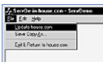
FIGURE 24.3 The File pop-up menu of the ServDemo IDR_SRVR_EMBEDDED menu as it appears at runtime, while the program is performing fully-opened editing of an embedded item contained in a document named House.con
