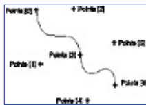
FIGURE 19.9 A curve consisting of two connected splines as drawn by the example code
