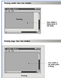
FIGURE 13.5 The areas in which the mouse cursor is confined for a drawing that's smaller than the view window, and for a drawing that's larger than the view window; in both cases, the cursor is confined within the intersection of the view window and the drawing (the dark shaded area)
