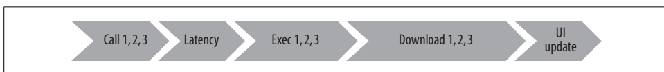
Figure 6-2. The batch call function combines multiple unit calls and executes them in one shot, which means there's only one request to server and one response to download
