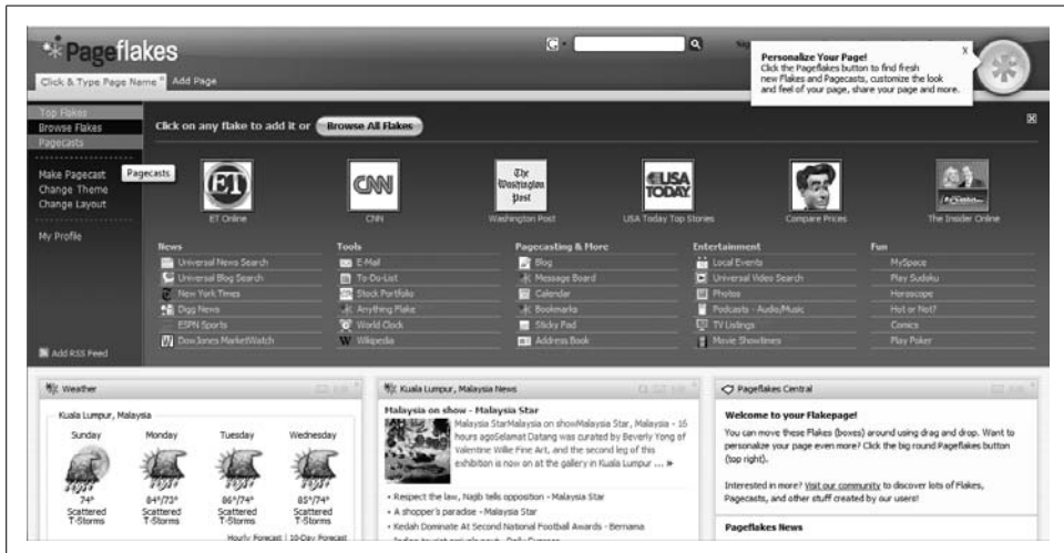
Figure 9-6. Loading large UI blocks on demand using XML HTTP. The black gradient box appears when you click the big round button on the top right; this whole area is loaded on demand.
