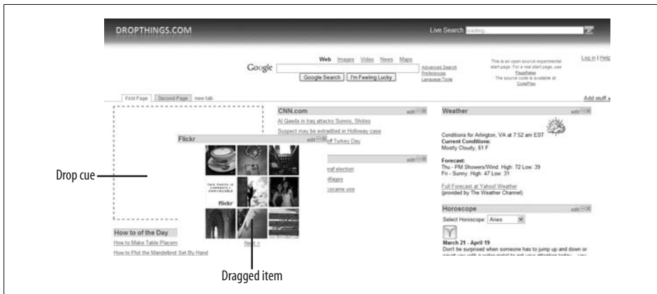
Figure 2-7. A page showing drag-and-drop behavior between columns and the drop cue that indicates where the widget can be dropped
