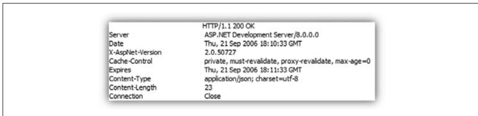
Figure 6-6. Incorrect HTTP response headers are generated from the web method when you try to produce the headers as documented
