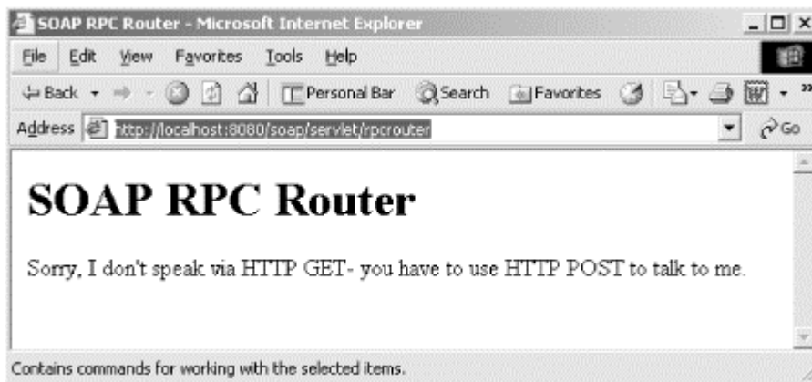
Figure 12-2. The RPC router servlet
