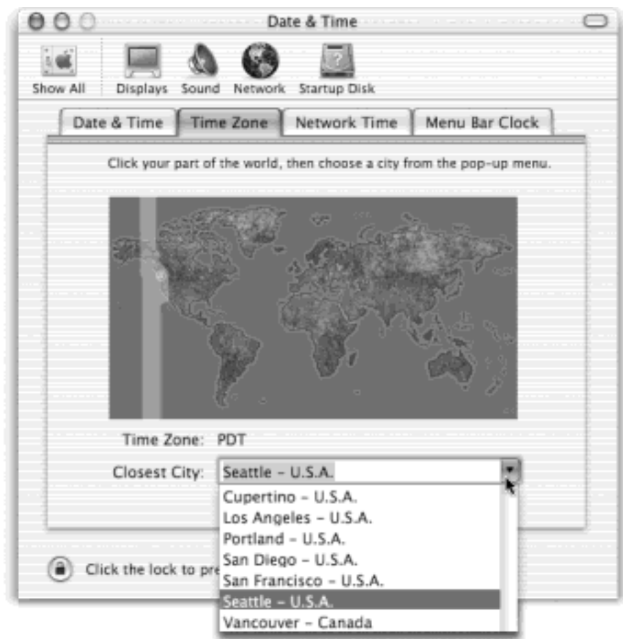
Figure 8-3. Setting the Time Zone is a two-step process. In the Time Zone pane, click on a section of the map to select a general region of the world, and then use the pop-up menu to specify your country within that region.
