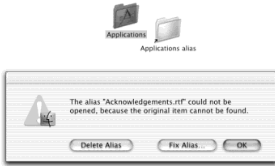
Figure 2-7. Top: You can identify an alias by the tiny arrow badge on the lower-left corner. (Longtime Mac fans should note that the name no longer appears in italics.) Bottom: If the alias can't find the original file, you're offered the chance to hook it up with a different file.
