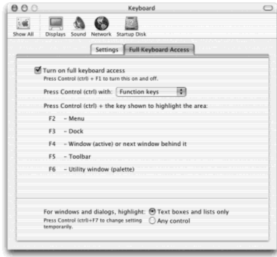
Figure 4-9. The Full Keyboard Access panel of the Keyboard control panel lets you specify how you'd like to control your menus and other Mac OS X interface elements without using the mouse.
