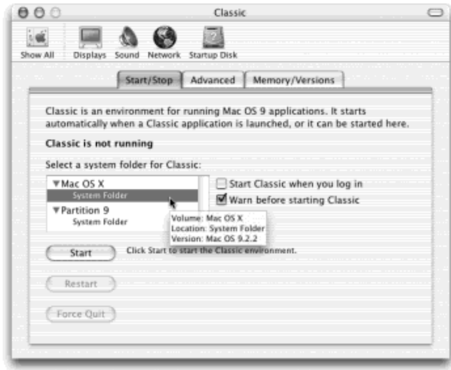
Figure 5-3. This preference panel lets you specify which Mac OS 9 System Folder takes over when you launch the Classic mode. If you point to a System Folder without clicking, a square balloon appears to identify its name, location, and system version.
