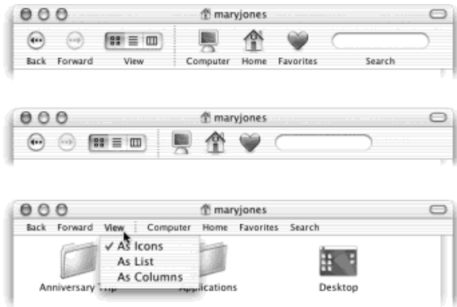
Figure 3-7. The Finder toolbar starts out with both picture and text buttons (top). But you may prefer to see only icons (middle) for greater horizontal compactness or only text (bottom) for greater vertical compactness. In that case, the trio of View icons turns into a single View pop-up menu, as shown here.
