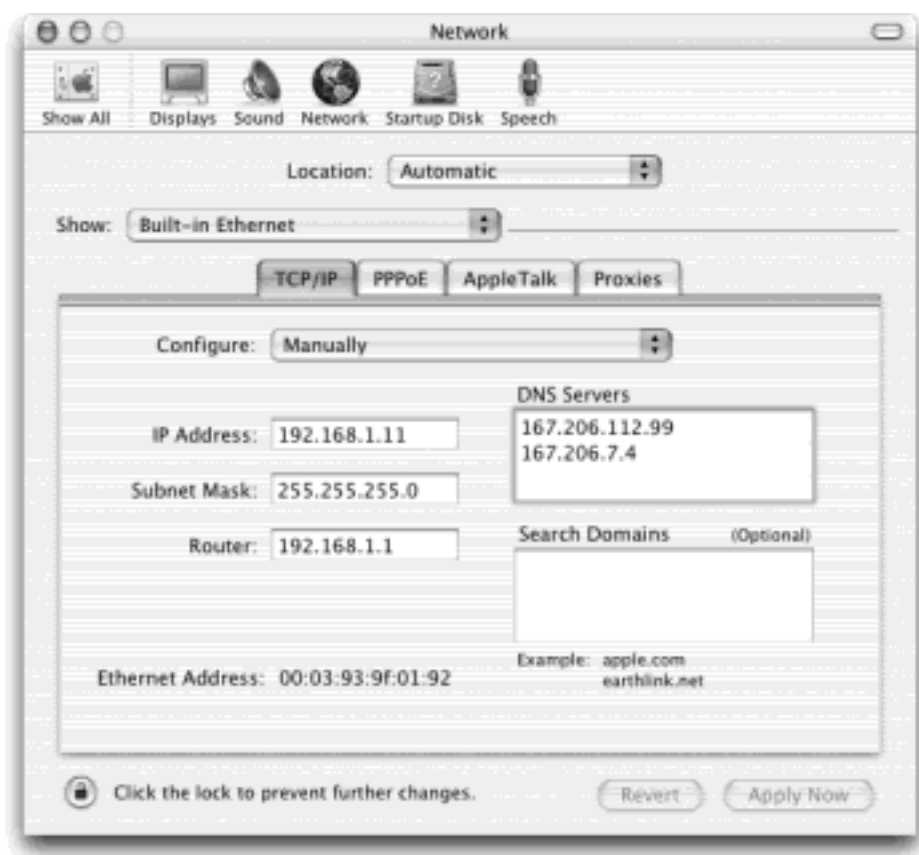
Figure 18-3. Don't be alarmed by the morass of numbers and periods—it's all in good fun. (If you find TCP/IP fun, that is.) In this illustration, you see the setup for a cable-modem account with a static IP address, which means you have to type in all of these numbers yourself, as guided by the cable company. The alternative is a DHCP server account, which fills most of it in automatically.
