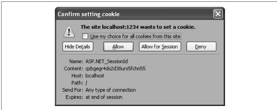
Figure 5-3. ASP.NET now sends out a session cookie on behalf of the page
