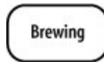
Figure 14-4. A rectangle with rounded corners and the name in the center is the most common way to draw a state
