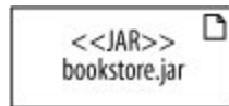
Figure B-1. An artifact with a JAR stereotype applied to it; this is an example of a stereotype you might see in a J2EE profile
