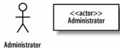
Figure 2-2. Requirement A.1 contains an Administrator actor that interacts with the system to create a blog account
