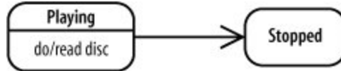
Figure 14-10. In this example, a transition is caused by the completion of internal behavior
