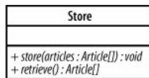
Figure 5-12. The store(..) and retrieve(..) operations do not now need to be implemented by the Store class
