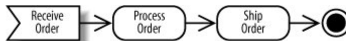
Figure 3-21. Starting an activity with a receive signal node: the receive signal node replaces the usual initial node
