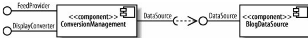
Figure 12-7. The ConversionManagement component requires the DataSource interface, and the BlogDataSource component provides that interface
