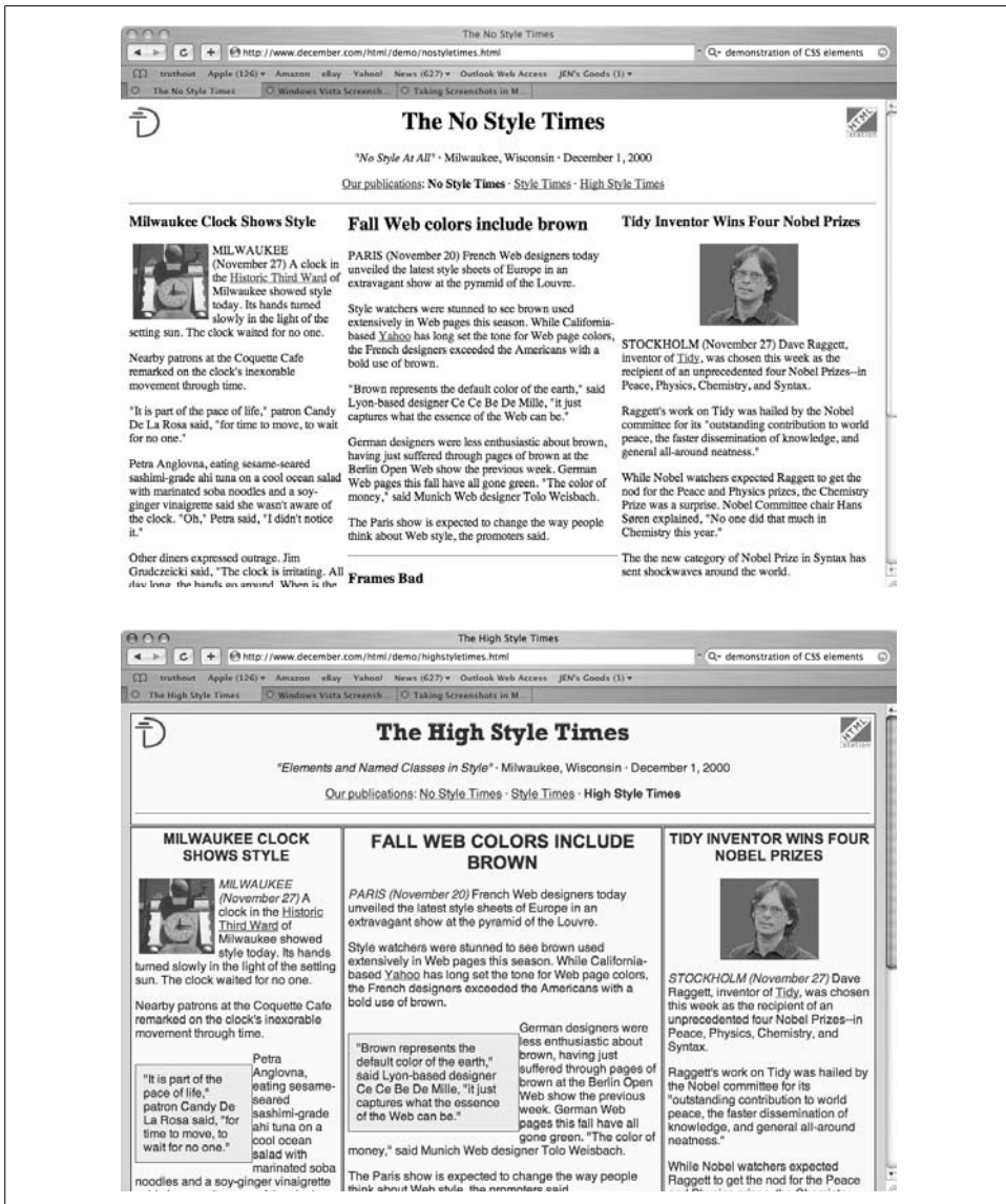
Figure 10-8. A web site as it displayed in earlier IE versions (top), and how it is supposed to look (bottom)
