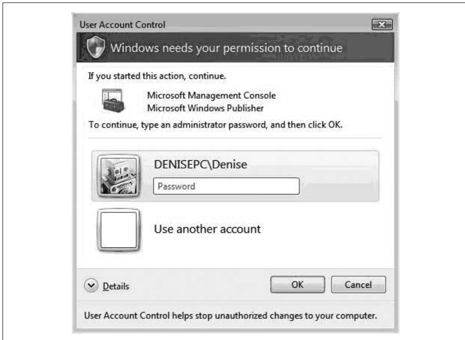
Figure 12-2. User Account Control requires regular users to provide credentials if they want to perform privileged functions
