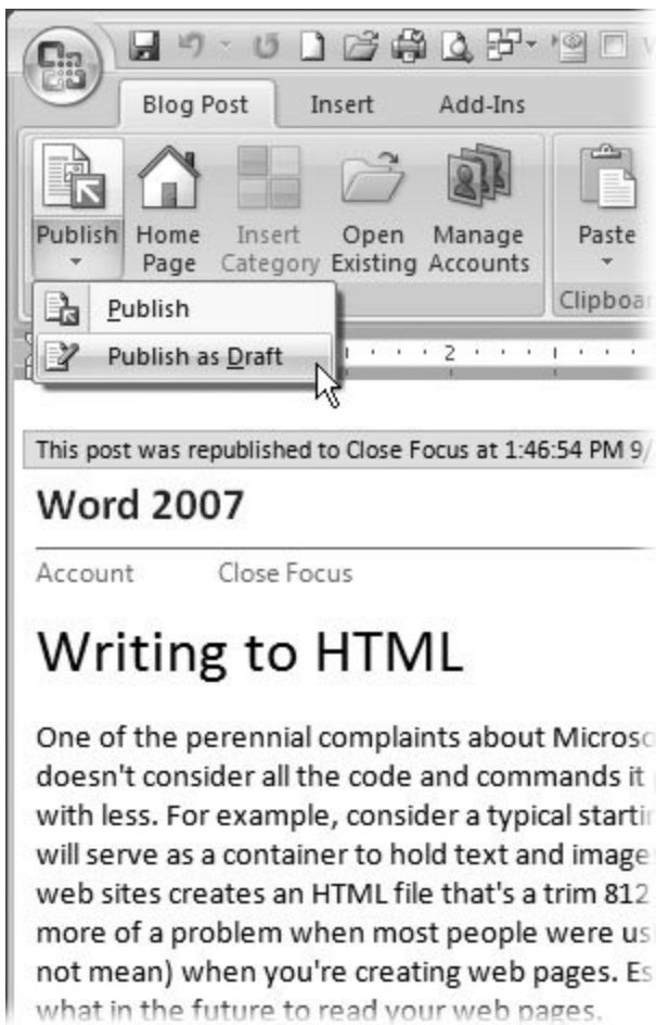
Figure 13-13. Click the Publish button to post your document as a blog entry. Click the Home Page button to open your blog in your Web browser. Use the Open Existing button to see previous blog entries and to open them for editing.
