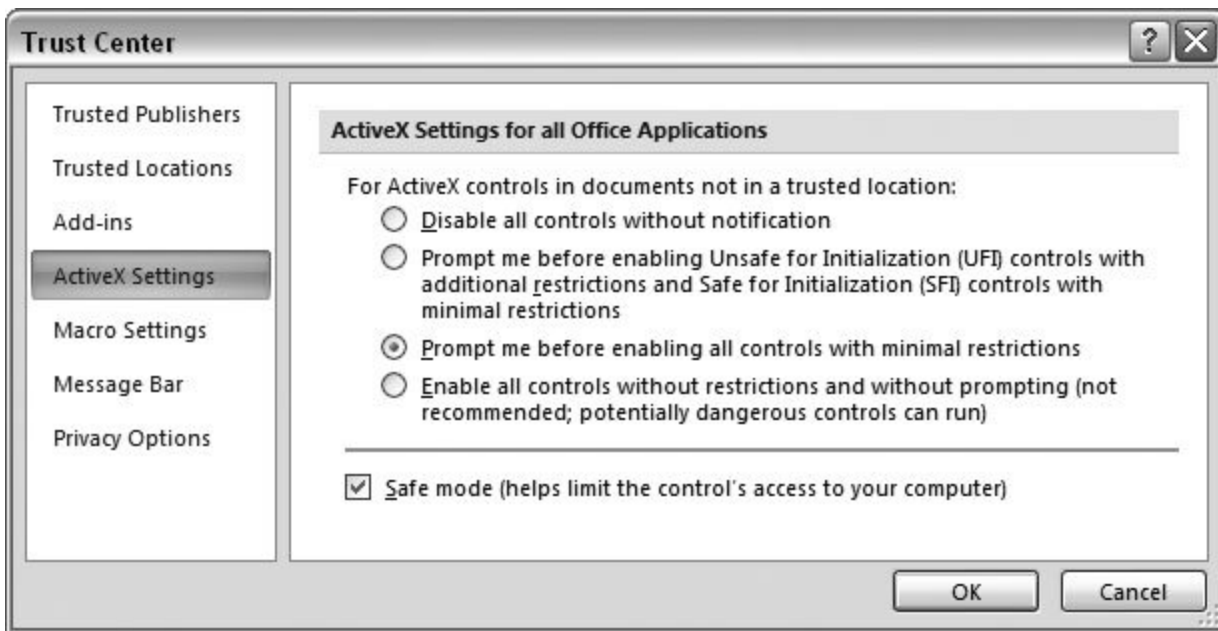
Figure 18-14. ActiveX controls are widgets like buttons or drop-down menus that can be embedded in Word documents. Use the settings in the Trust Center to rein in the controls, so that they can't run programs without your knowledge and consent.
