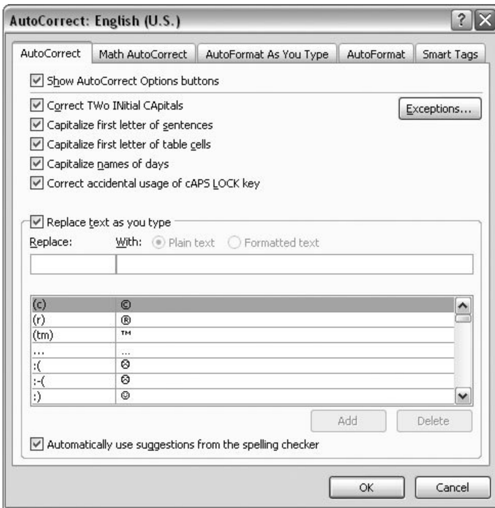
Figure 6-12. AutoCorrect likes to mess with your words as you type them. Fortunately, you can rein it in using this box. Use the checkboxes at the top to turn on (or off) AutoCorrect's fixes for some common typos. The box at bottom lists the changes AutoCorrect makes. By adding your own replacement pairs to this list, you can even use AutoCorrect as if it were AutoText.
