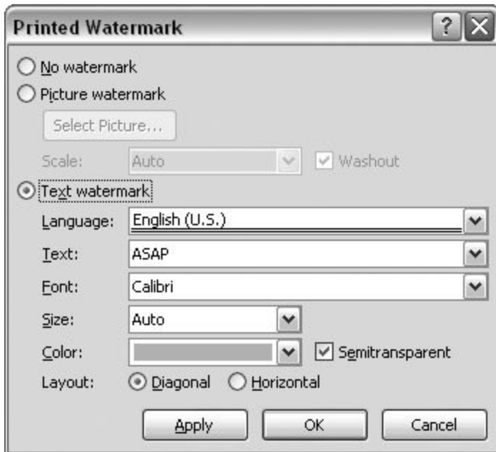
Figure 3-7. Using the Printed Watermark box, you can brand your document with a word of your choice. Simply type it in the Text box. Use the Font, Size, Color, and Layout options to change the text's appearance.
