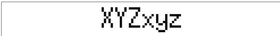
Figure 10-1. Enlargement of a monochrome font showing aliasing; note the staircase effect on diagonal lines.
