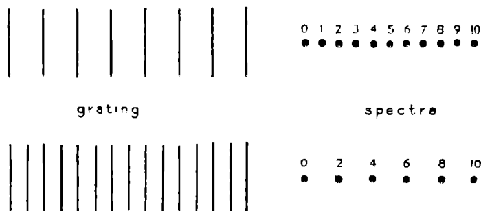
FIG. 70. Effect of doubling the number of lines in a grating is to eliminate odd order spectra.
