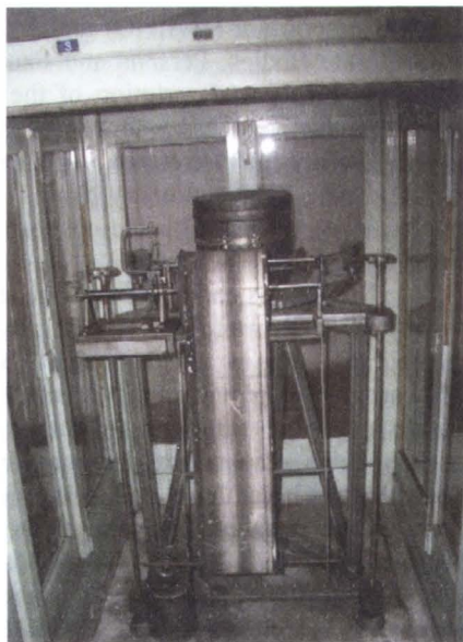
The Wiechert horizontal component seismograph (c. 1908)
