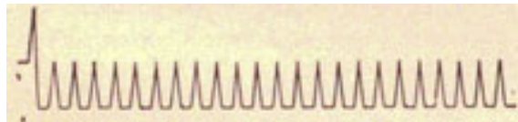
Figure 4 SF-5. Pattern for calibrating 2,000-yard range on 48,000-yard scale.
