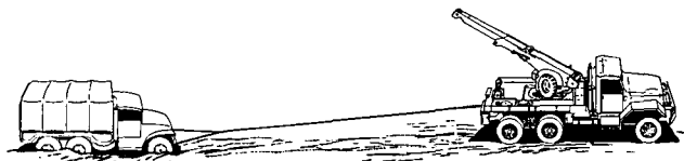
Figure 100. Recovering mired truck with a wrecker truck.
