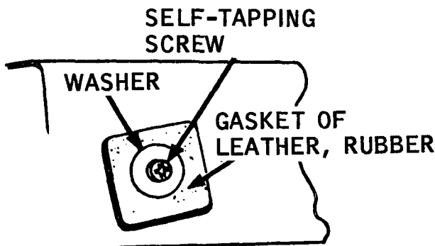
Figure 78. Pinhole-size leaks in fuel tanks.
