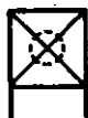
BORESIGHTING AND ZEROING TARGET FOR THE MAIN GUN, USED TO BORESIGHT COAX MACHINEGUN.
