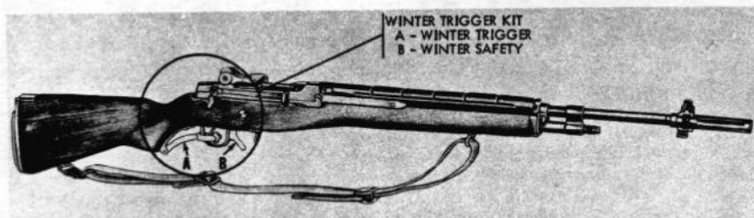
Figure 60. M14 rifle with winter trigger kit.
