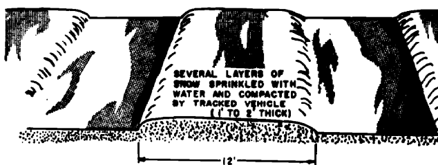
Figure 5-7. Road reinforced with snow.
