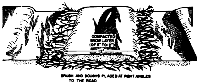
Figure 5-8. Road reinforced with brush and snow.
