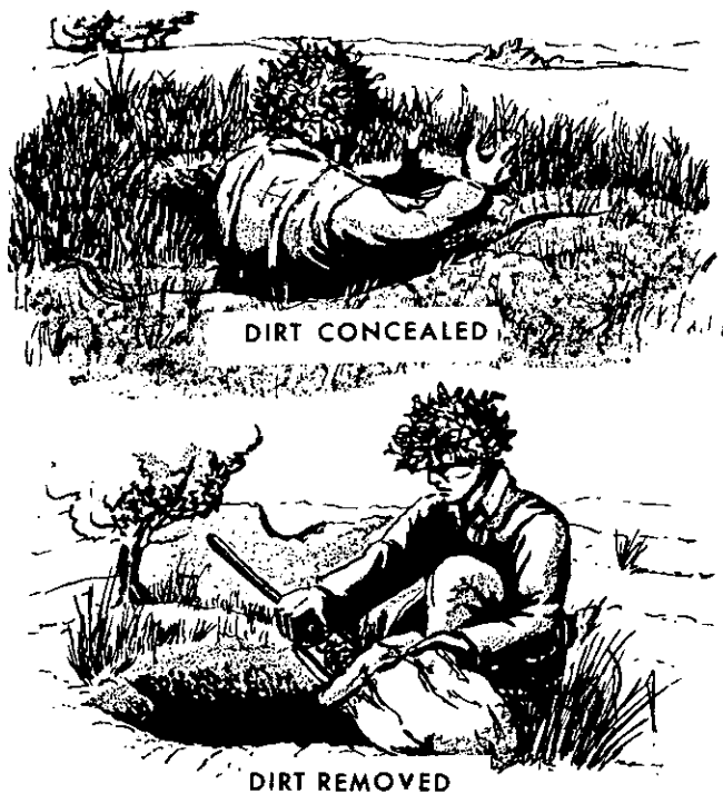
Figure 2-3. Disposal of soil.
