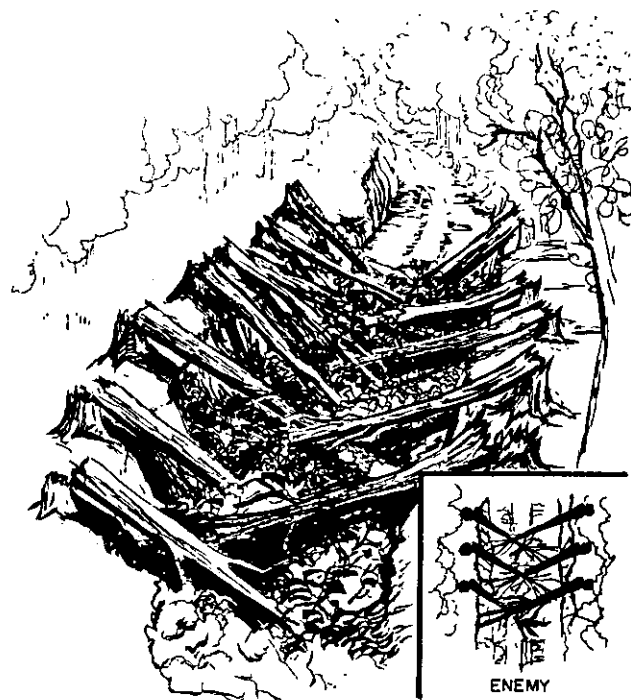
Figure 7-8. Abatis used as roadblock.
