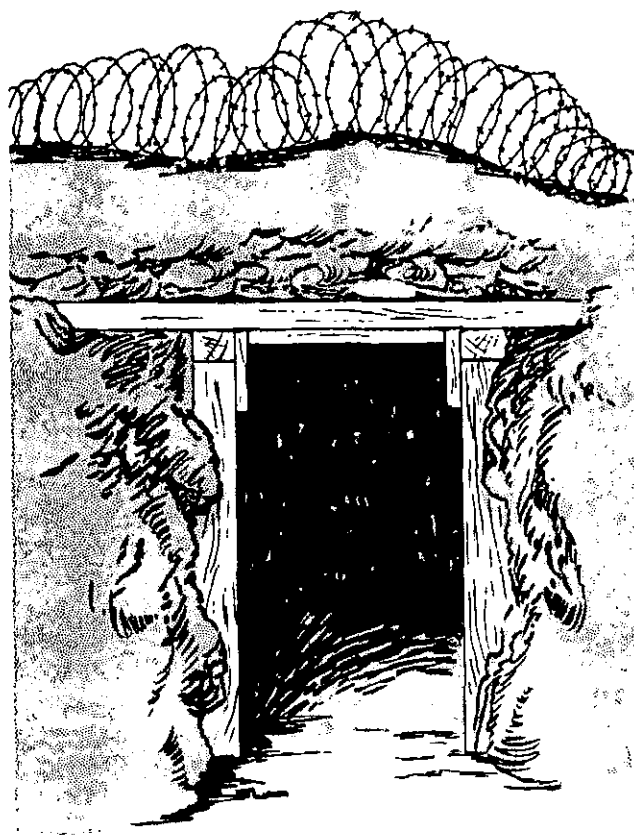
Figure 6-2. Protective wire on top of overhead cover.
