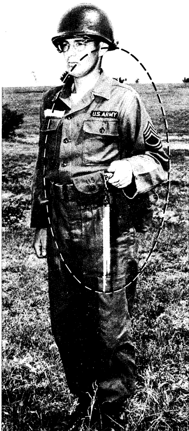
Figure 32. Ventilation of psychrometer.
