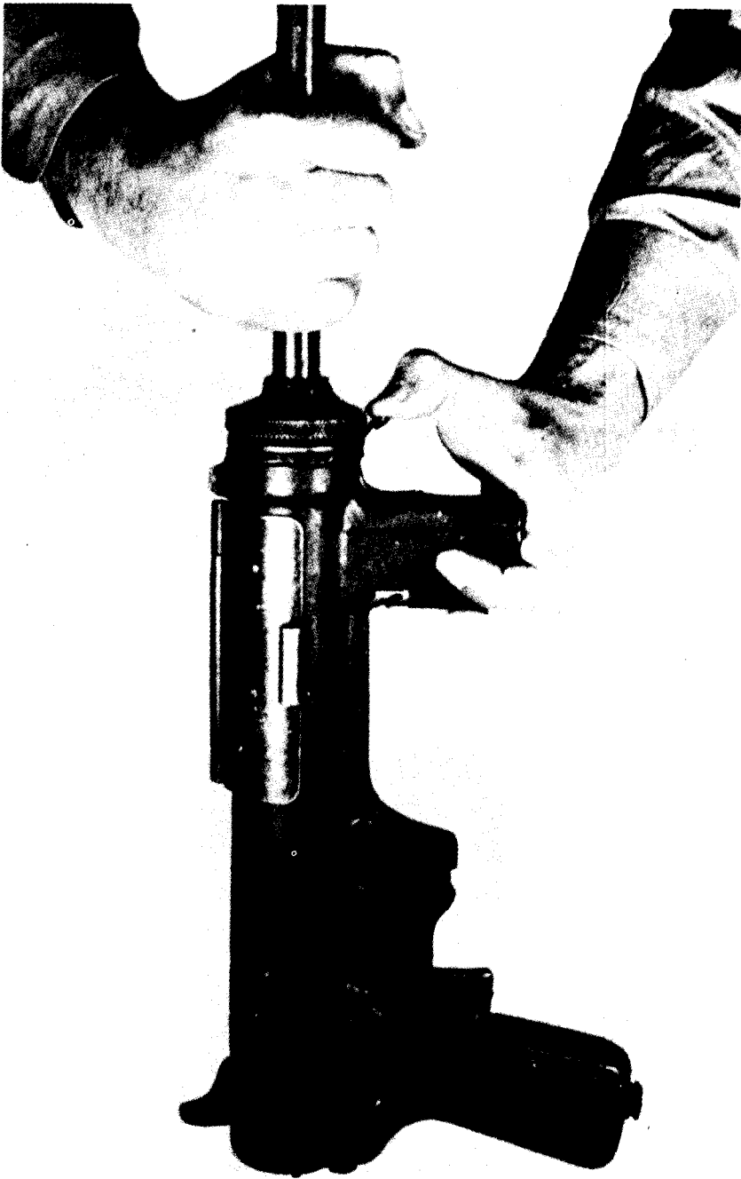
Figure 9. To remove the barrel, make sure the bolt is forward, depress the barrel ratchet, and unscrew the barrel. Do not allow the barrel ratchet to contact the notches in the barrel collar when removing or replacing the barrel.
