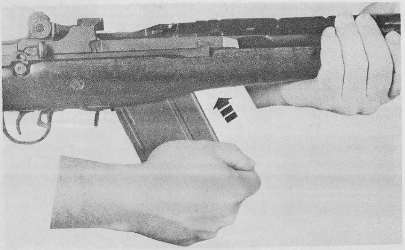
1 Figure 29. Loading the magazine into the rifle.
