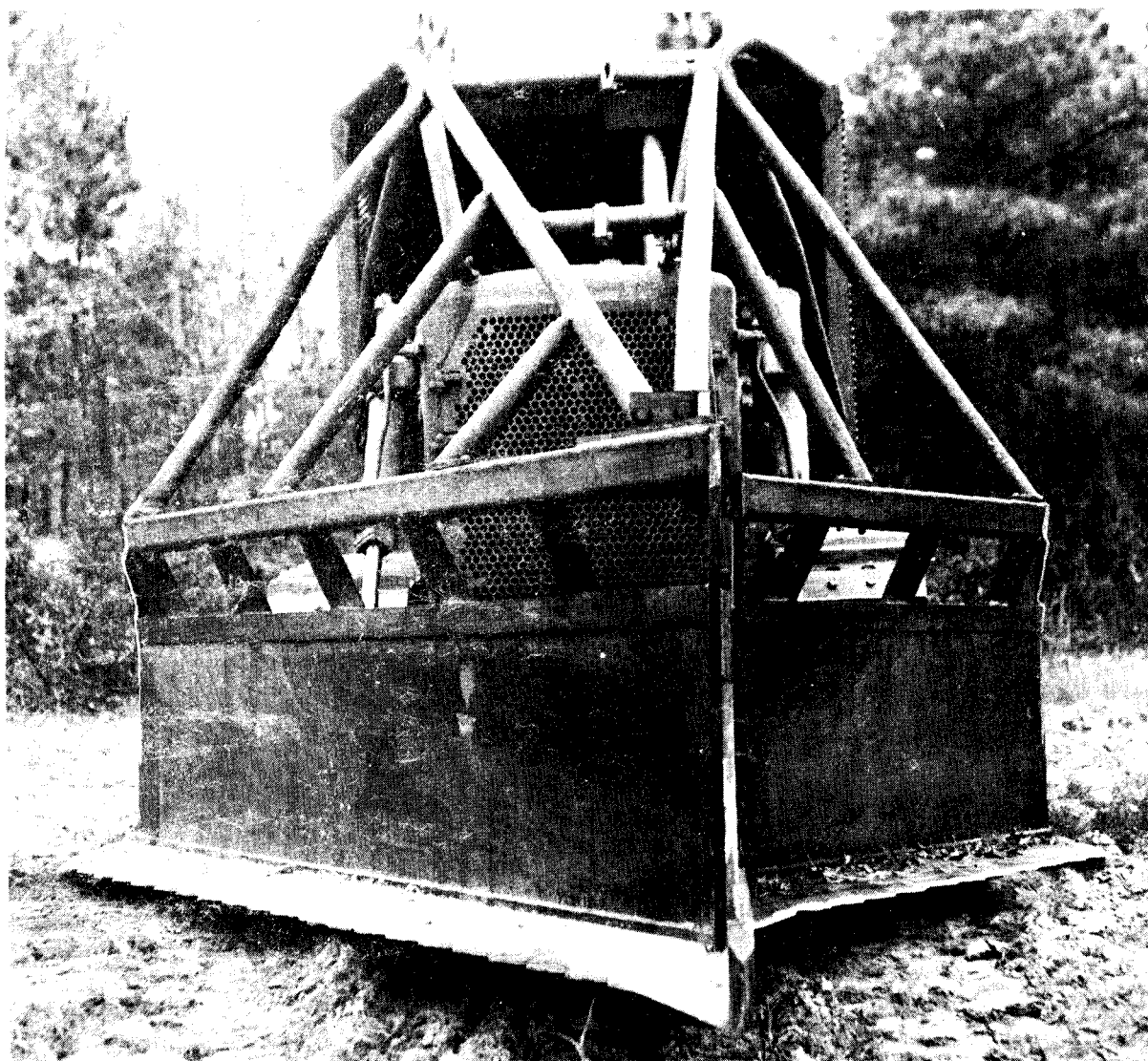
Figure 3-19. "V" type clearing blade with serrated cut edges and a center-mounted splitter.
