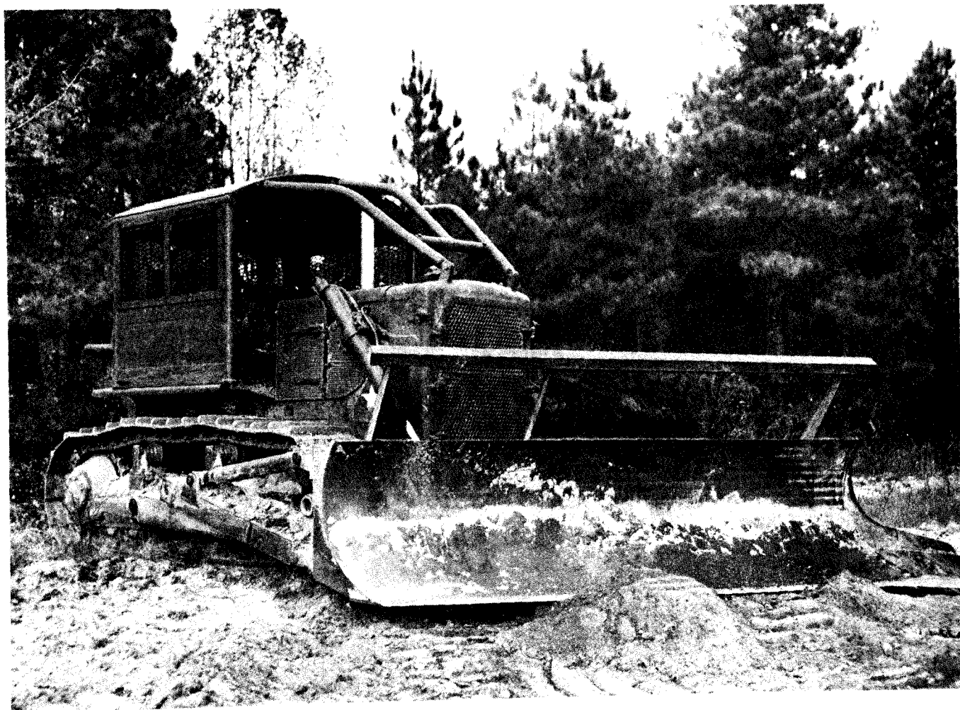
Figure 3-17. Rome K/G clearing blade.
