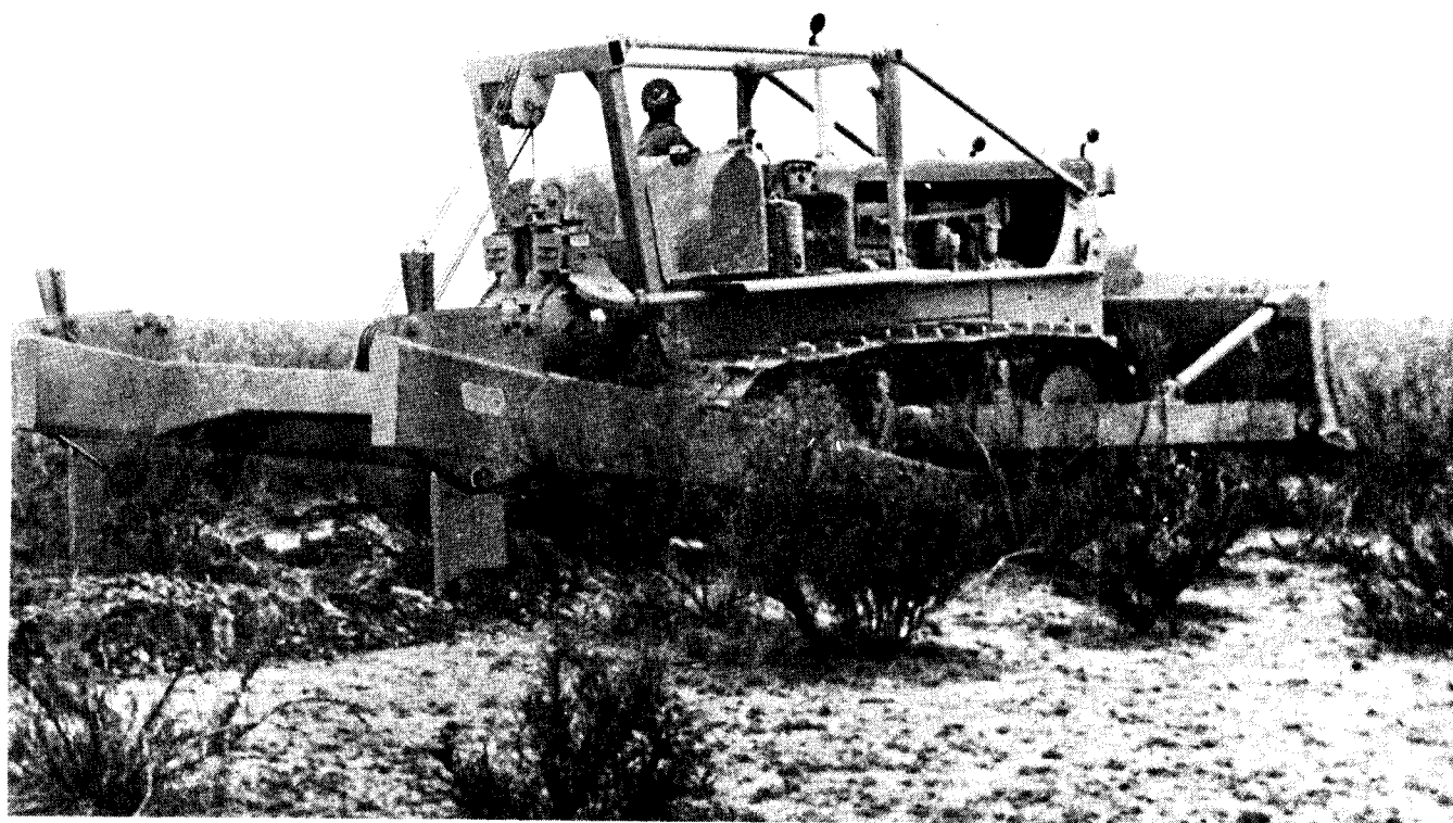
Figure 3-7. Trunnion-mounted root plow.
