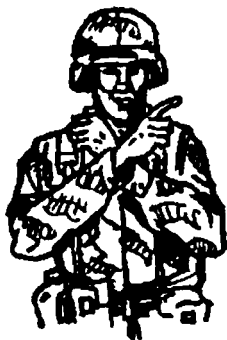
Figure 2-19. NEUTRAL STEER (track vehicles).
