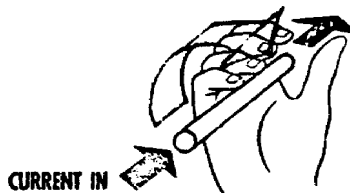
Figure 17. Application of Right-Hand Rule.
