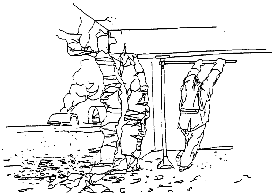
Figure 7.45. Shoring Jack Installation.
