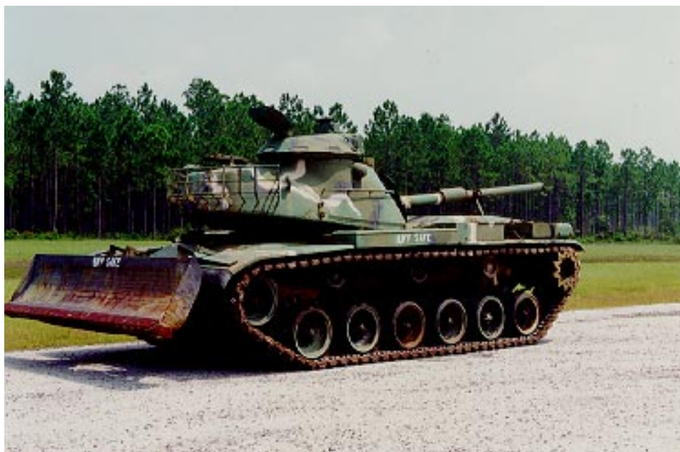
Figure 4.11. M-60 Mass Ordnance Clearance Vehicle.
