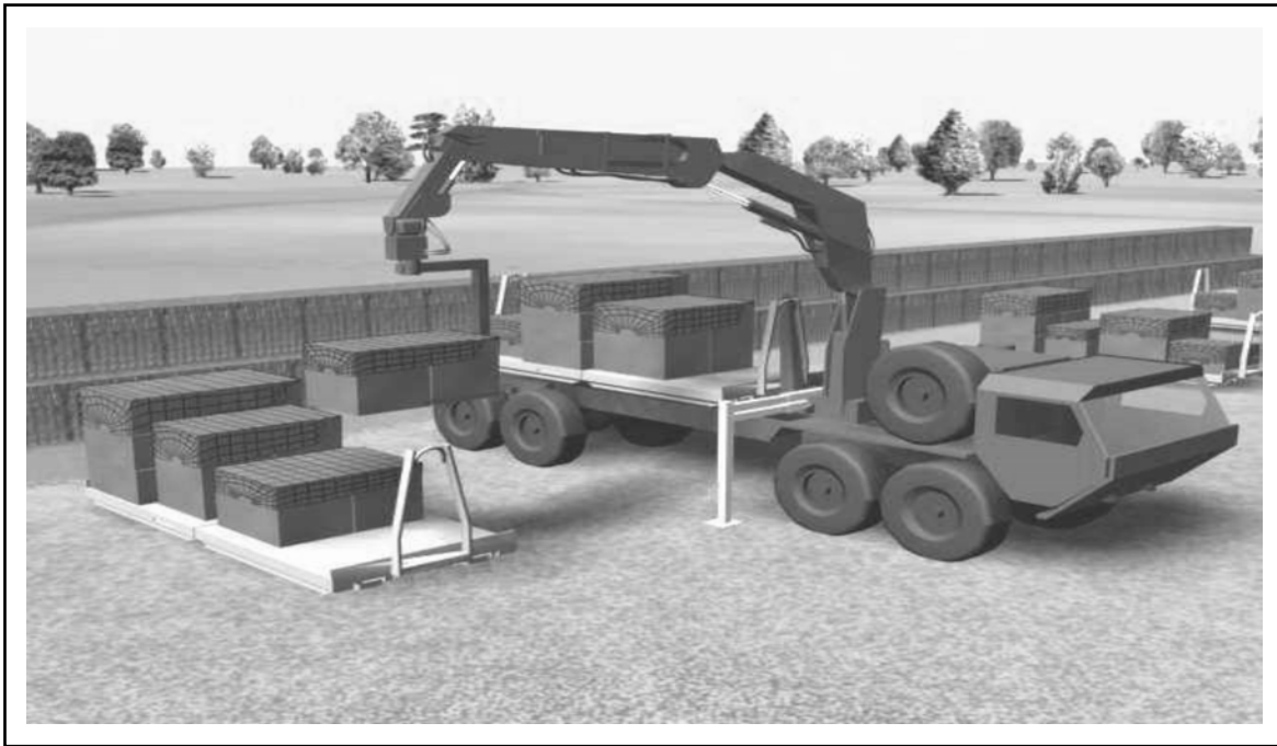
Figure 3-6. The FTTS with the Intelligent Load Handling System
