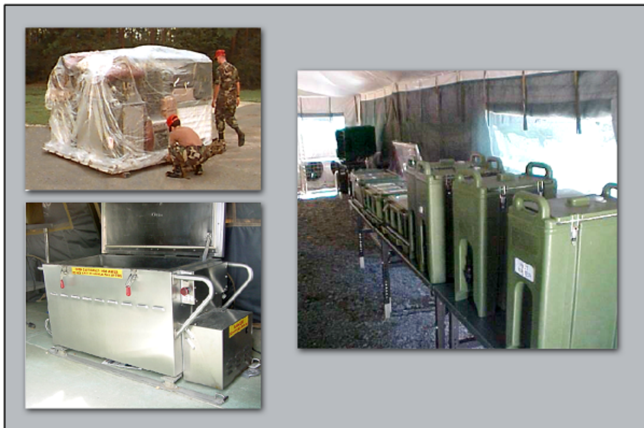
Figure 19. SPEK Pallet As Deployed with TEMPER Tent.
