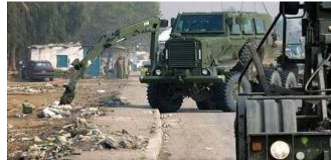
South-African developed Buffalo mine clearing vehicle probing & clearing mines & IEDs in Iraq
