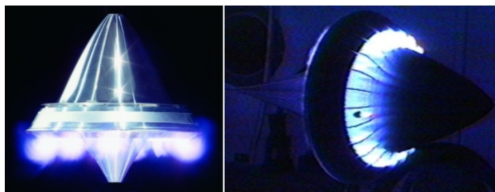
Figure 3.2.—Lightcraft plasma engine pulsing in 1-bar laboratory air (photographs by J.E. Shryne, III). Left: 14.7-cm-diameter #200 vehicle. Right: 23-cm #100 vehicle.
