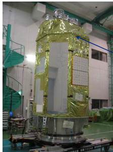
MLI covering the outside of a spacecraft
