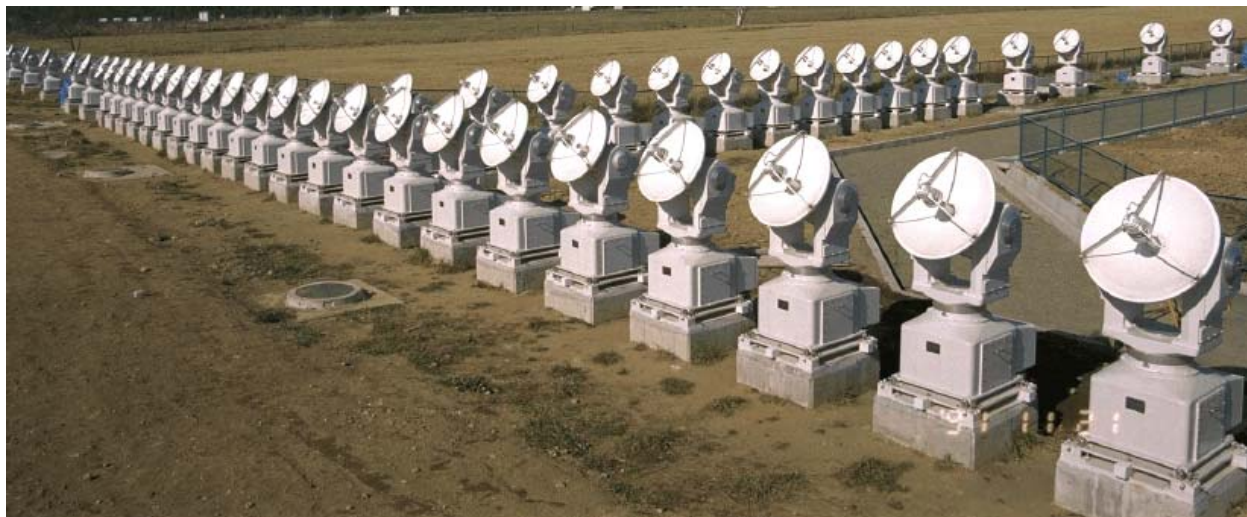
Figure D.18.—84-element Nobeyama Radioheliograph array for 17 GHz and 34 GHz reception. Each antenna is 80cm in diameter (Ref. 13).
