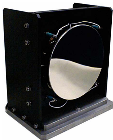
Figure 3.117.—Left: 12-cm-diameter fast-steering mirror for high-power laser applications (image courtesy of ATA; used with permission). A 30-cm-diameter model features >1-kHz open-loop bandwidth, >300 rad/s 2 angular acceleration, <0.2-μm surface accuracy, and ±8-mrad mechanical travel with <10-μrad (2-arcsec) pointing accuracy. Right: YAL-1A ABL prototype in flight, 1.5-m telescope, megawatt-class 1.3-μm laser with undisclosed range .
