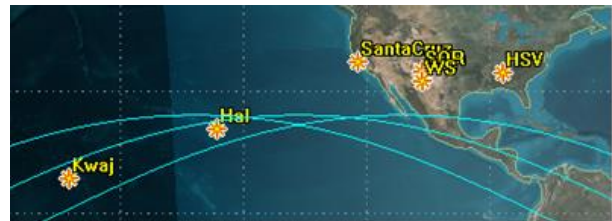
Fig. 1 The LightSail 2 ground track is well below the ability of most sites in the continental United States to achieve sufficient laser dwell time.
