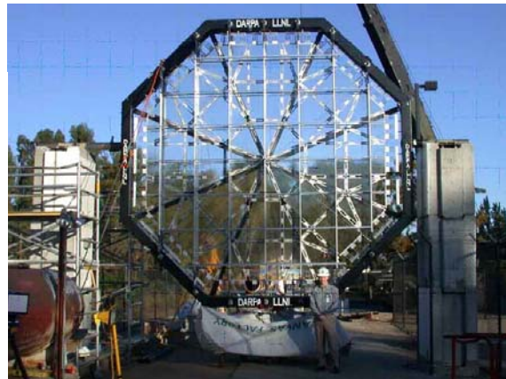
FIGURE 4. Five meter diffractive optic demonstrated at LLNL. Optic is made with 700 \mu\text{m} glass. To reach \ll 1 \text{ kg/m}^2 , a lens would have to be made from even thinner ( \sim 100 \mu\text{m} ) panels, but such material is commercially available in meter-sized panels, and can be patterned and handled (we have wrapped 75 \mu\text{m} sheets around coke cans) with the same techniques.
