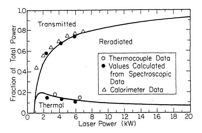
Figure 3 Experimental and Numerical Model Results for Global Absorption and Thermal Efficiency as a Function of Laser Power
