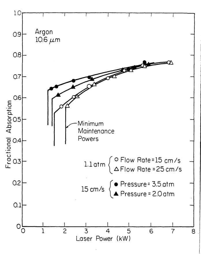
Figure 4 Global Absorption Data Taken at High Gas Pressures and Flow Velocities
