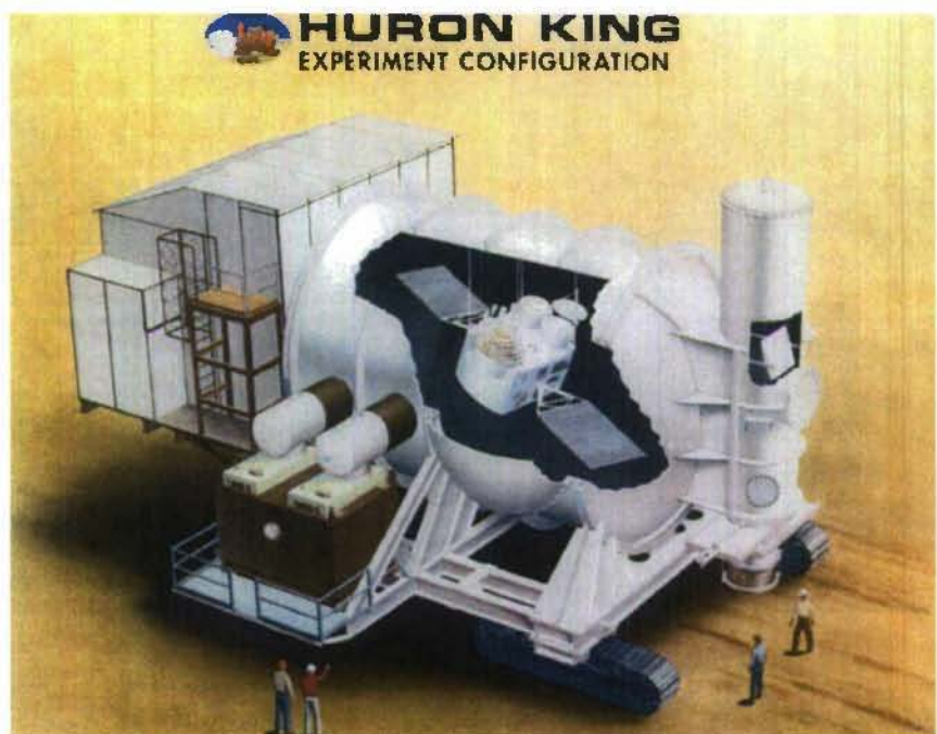
Figure IV.3. Experimental chamber containing STARSAT in the HURON KING event.
