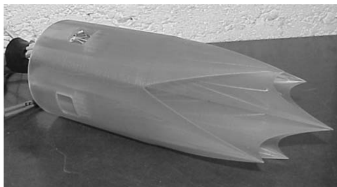
Figure 2.31: Final modular intake shape (Matthews & Jones, 2006).
