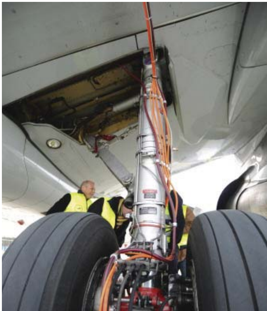
The GreenTaxi system provides 11,000 Newton-metres of torque power. Test data is being evaluated prior to deciding whether or not to develop a prototype.
