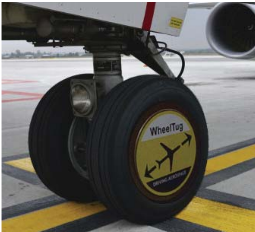
The wheelTug system uses two electric motors in the nosewheel. These are electrically powered, deriving power generated by the aircraft's APU.
