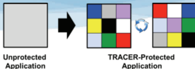
Figure 1: TRACER frequently randomizes the sensitive internal data and layout of the application after every possible leakage point.
