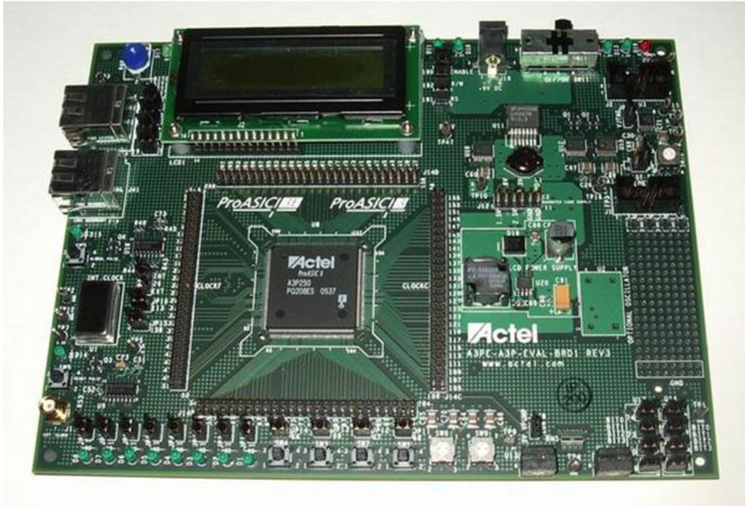
The ProASIC3 evaluation board hosts an A3PE600 device in a PQ208 package. It is programmed using the USB-based FlashPro3 JTAG emulator. Most of the on-board peripherals are jumper selectable, allowing easy reconfiguration.
