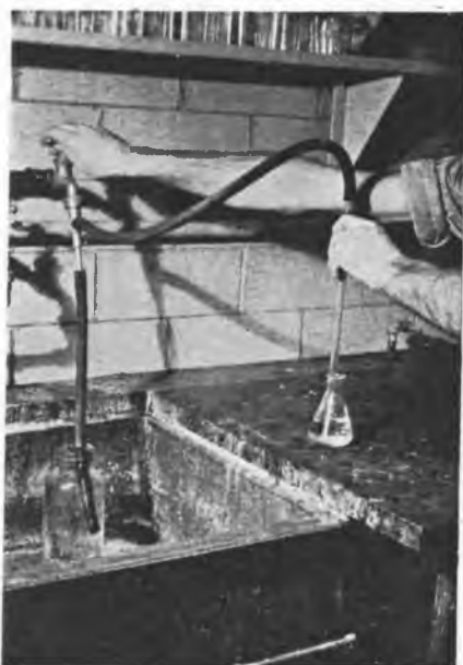
Courtesy Hercules Powder Co. Figure 11. Water-aspirating line for filling pipette. (See paragraph 68.)
