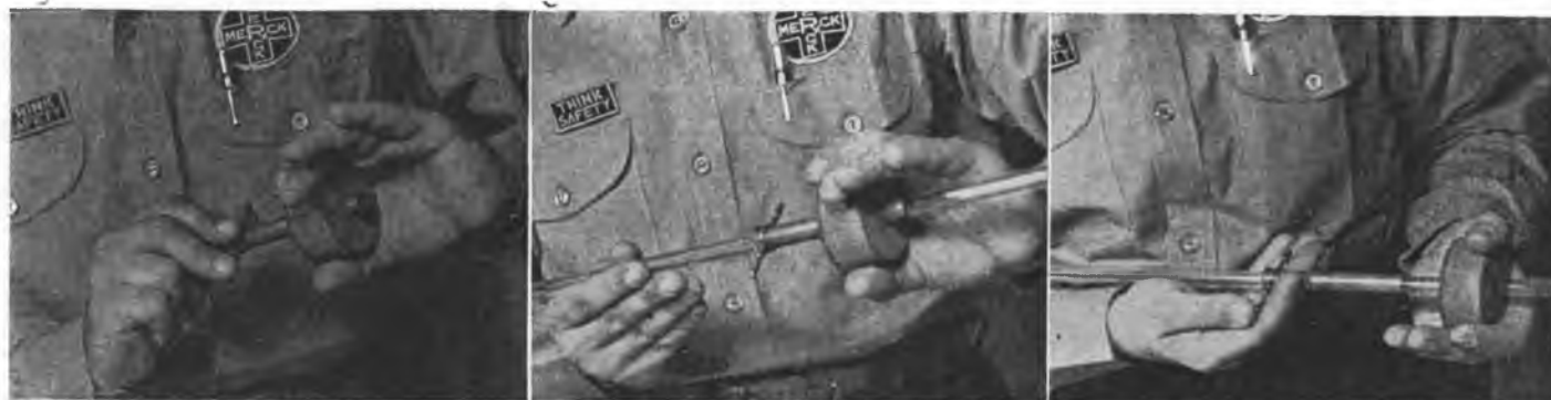
Figure 8. A safe method for inserting glass tubes in stoppers. Left: Bore hole in stopper; Center: Position glass tube through borer; Right: Remove borer. (See paragraph 63.)
