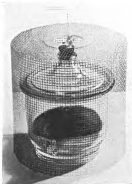
Courtesy Hercules Powder Co. Figure 9. Before a vacuum desiccator is evacuated, it should be placed under a 4-mesh galvanized screen basket. As a substitute, a wood box may be used. (See paragraph 66.)
