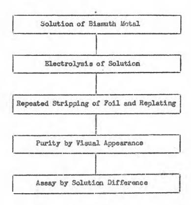
Electrolysis of the original solution was a very long, time-consuming process. Removal of the original plate by an acid leach and replating was sometimes repeated as much as ten times. Repetition of this procedure ceased when a firmly adhering, metallic-like plate was obtained.
