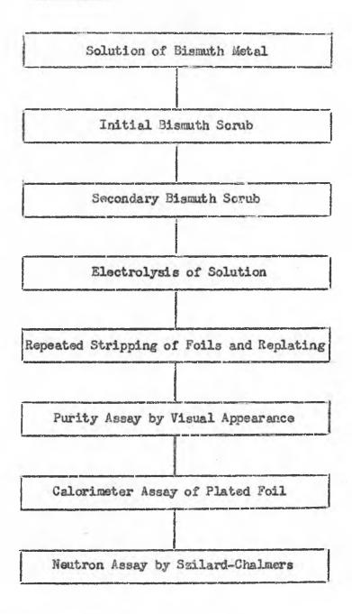
The two bismuth scrubs introduced here gave increased purification, a more suitable bismuth-polonium ratio by a factor of 100,000 and markedly decreased the stripping and replating operations. The calorimeter assay was made the official assay value for inter-site shipments. The neutron assay gave the first rough indication of the purity obtained.
