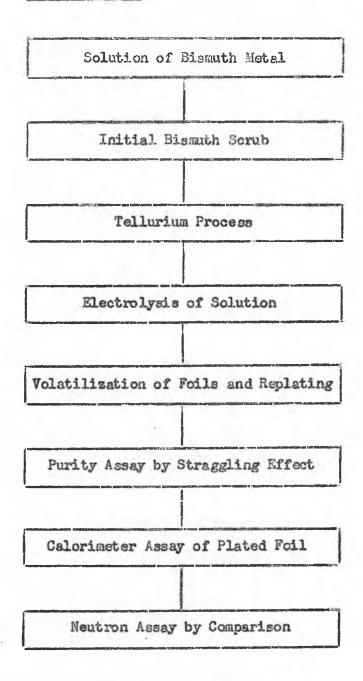
The tellurium process produced for the first time a solution for plating that was comparatively free from foreign metallic ions.
