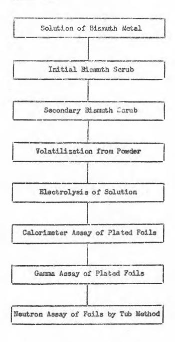
The development of a method for the direct volatilization of polonium from bismuth powder resulted in much greater purification and lightened the load carried by the Electroplating Group to a considerable extent. The gamma assay of the plated foil, when compared to the calorimeter assay of that foil, gave a very good indication of the purity of the plated polonium.
