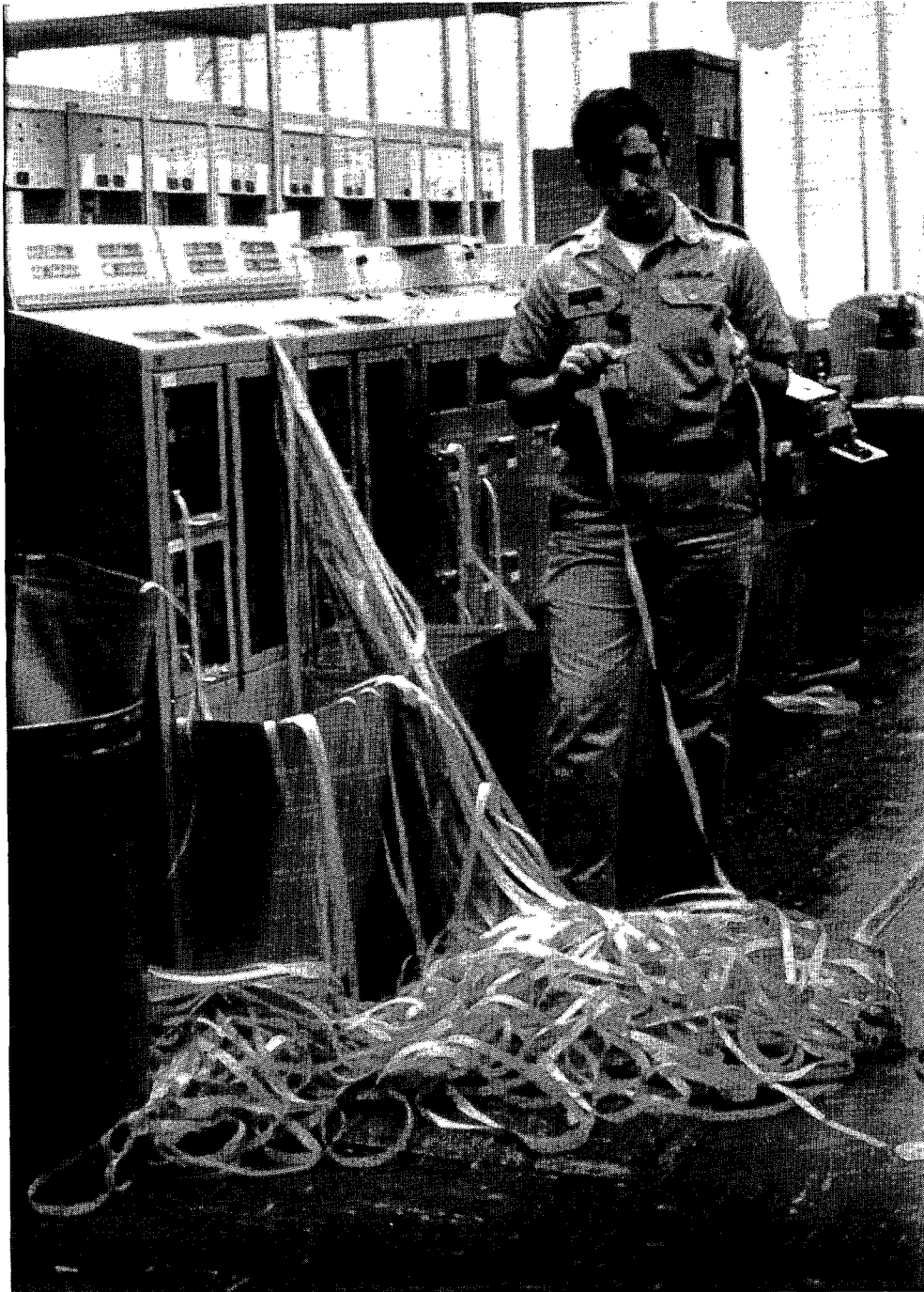
Comm Center, 1960s. Lacking a digital switch, Criticomm centers continued to be overwhelmed by five-level tape and manual processing.
