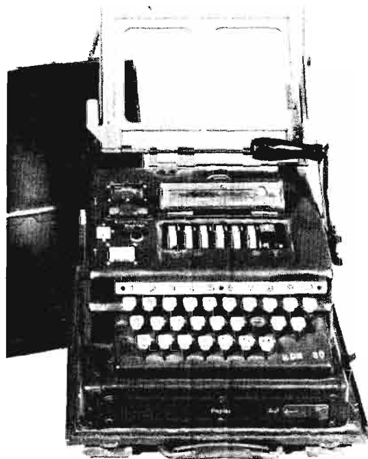
Menzer Device SG-41. A successful encipherment system, but of limited use due to its heavy weight.
