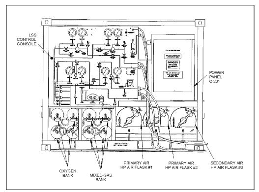
Figure 22-10. Fly Away Recompression Chamber Life Support Skid.
