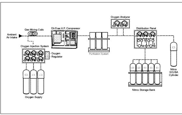
Figure 10-3. Nitrox O<sub>2</sub> Injection System.
