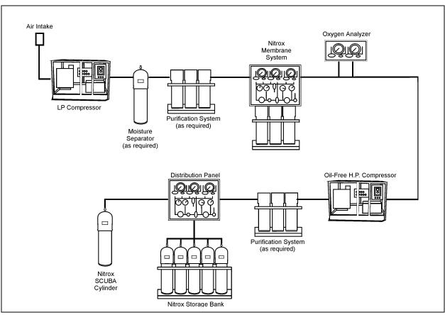
Figure 10-4. LP Air Supply NITROX Membrane Configuration.
