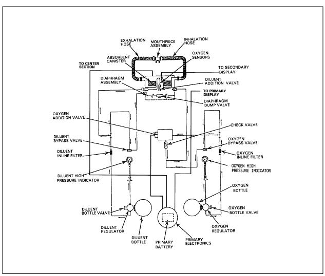
Figure 17-2. MK 16 MOD 0 UBA Functional Block Diagram.
