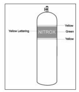
**Figure 10-2.** NITROX Scuba Bottle Markings.
