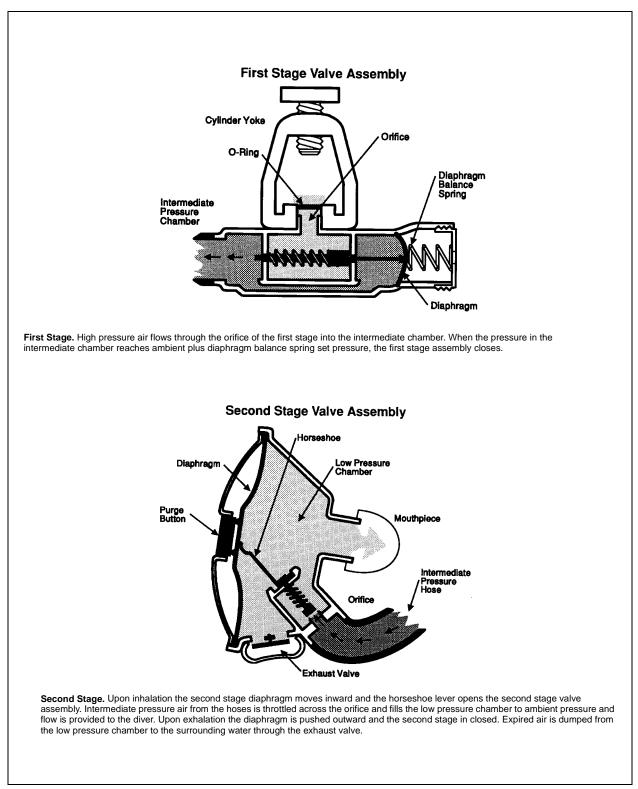
Figure 7-1. Schematic of Demand Regulator.
