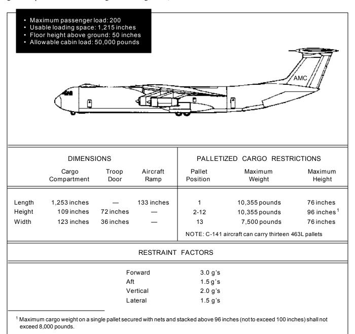
Figure 2-18. Characteristics of C-141 aircraft
