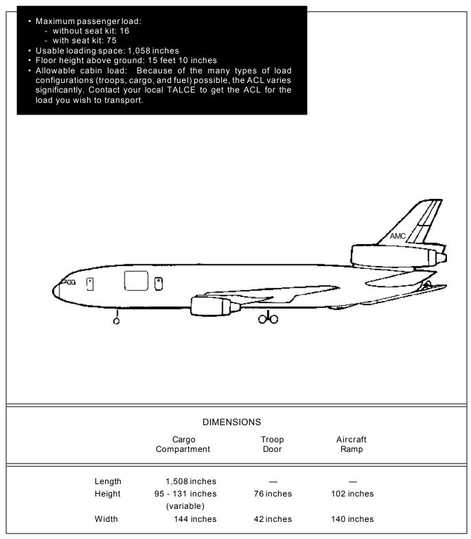
Figure 2-20. Characteristics of KC-10A aircraft
