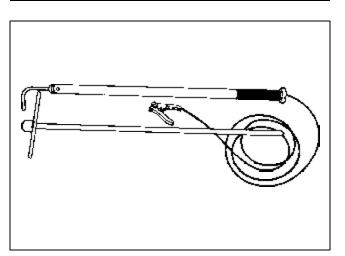
Figure 2-11. Static electricity discharge probe
