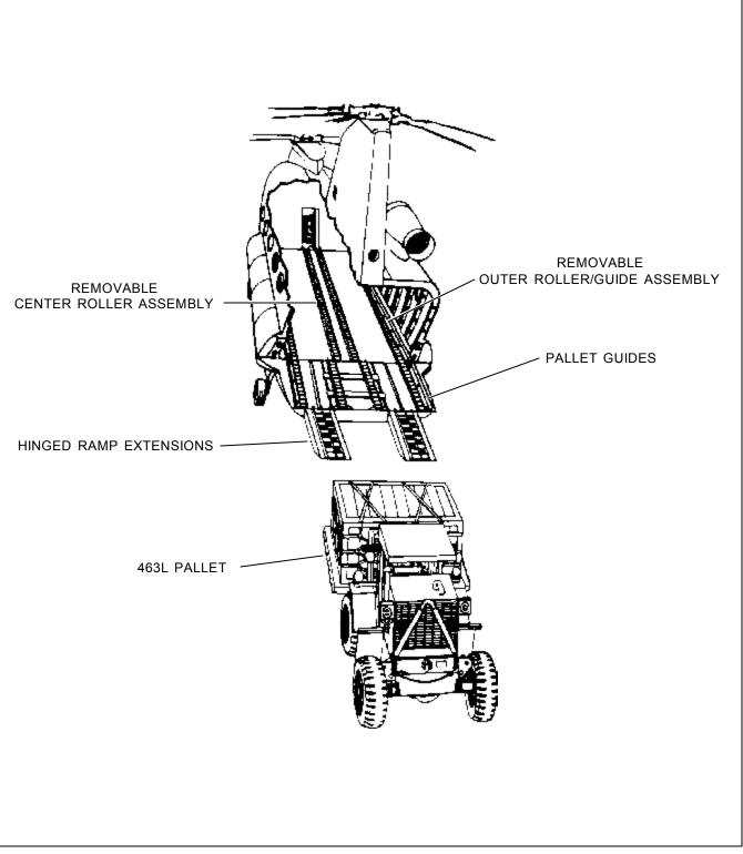
Figure 2-15. HICHS installed in a CH-47 helicopter
