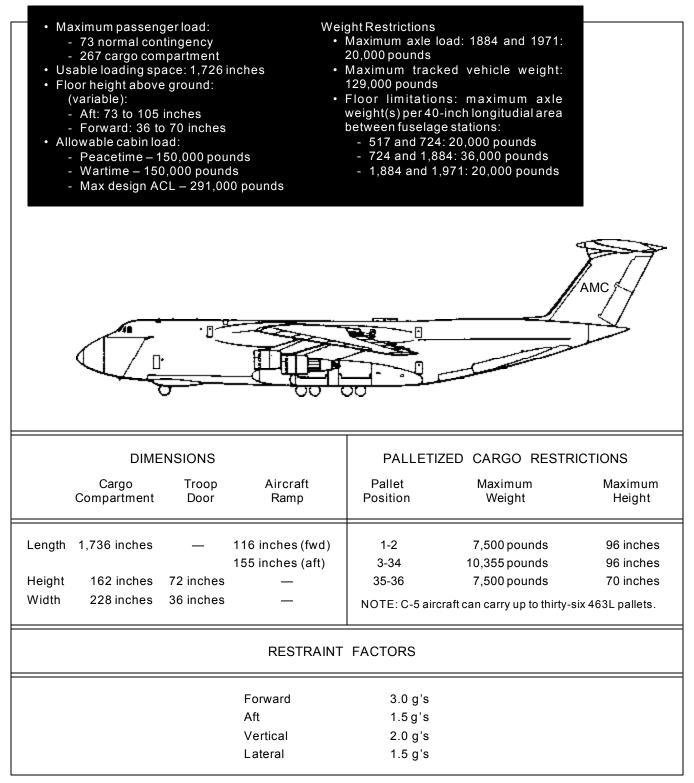
Figure 2-19. Characteristics of C-5 aircraft
