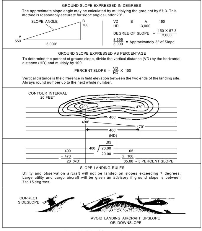
Figure 2-3. Determining ground slope
