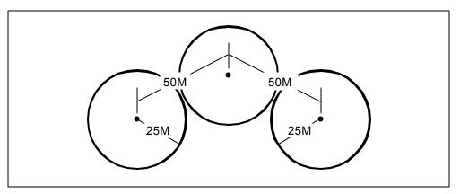
Figure 2-2. Size 3 aircraft landing zone for V-formation
