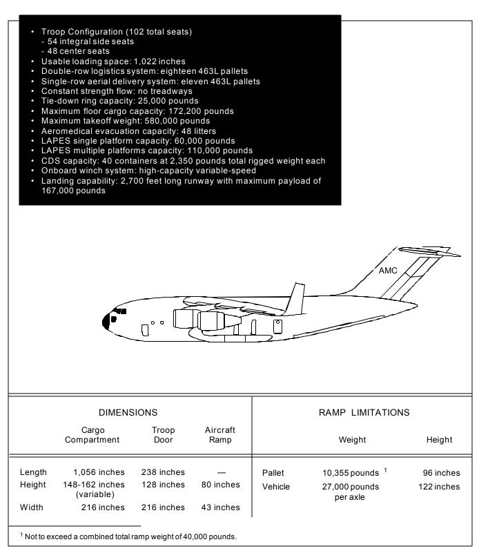
Figure 2-21. Characteristics of C-17 aircraft
