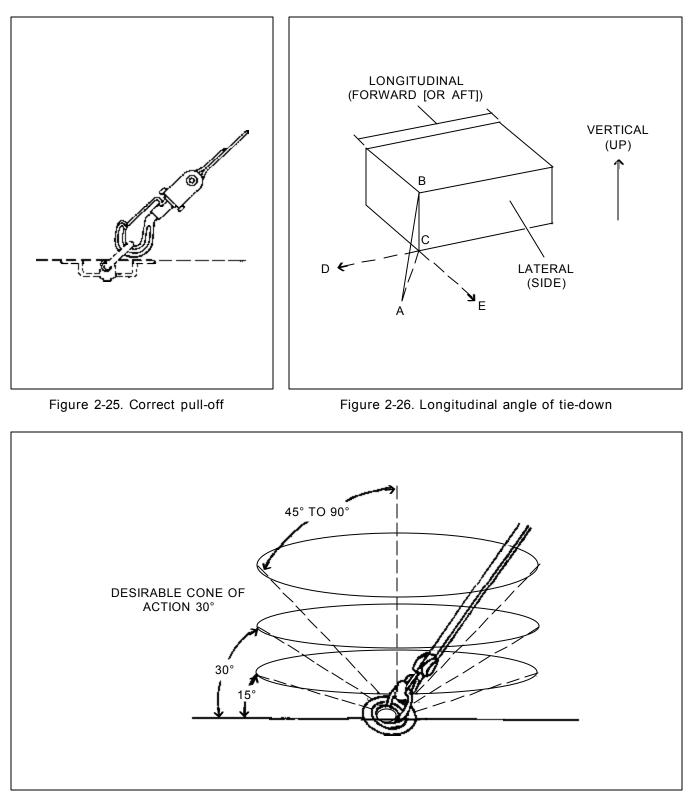
Figure 2-27. Vertical angle of tie-down
