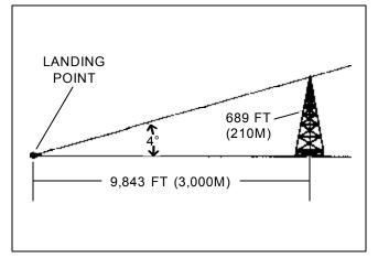
Figure 2-5. Maximum angle of approach (nighttime)
