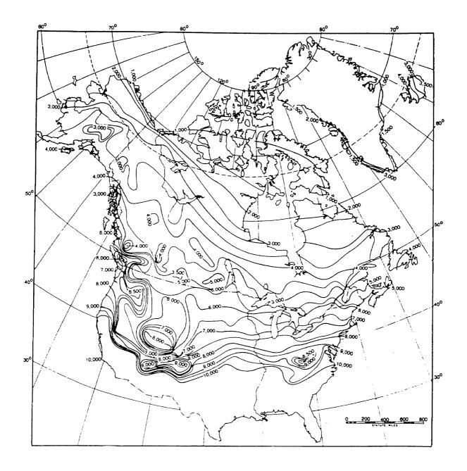
Figure 12-5. Distribution of mean air thawing index values for pavements in North America (0).
