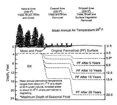
Figure 12-8. Permafrost degradation under different surface treatments.
