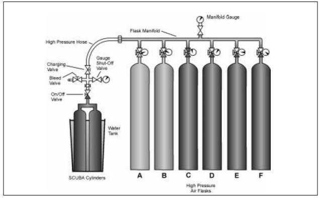
Figure 7-7. Cascading System for Charging Scuba Cylinders.
