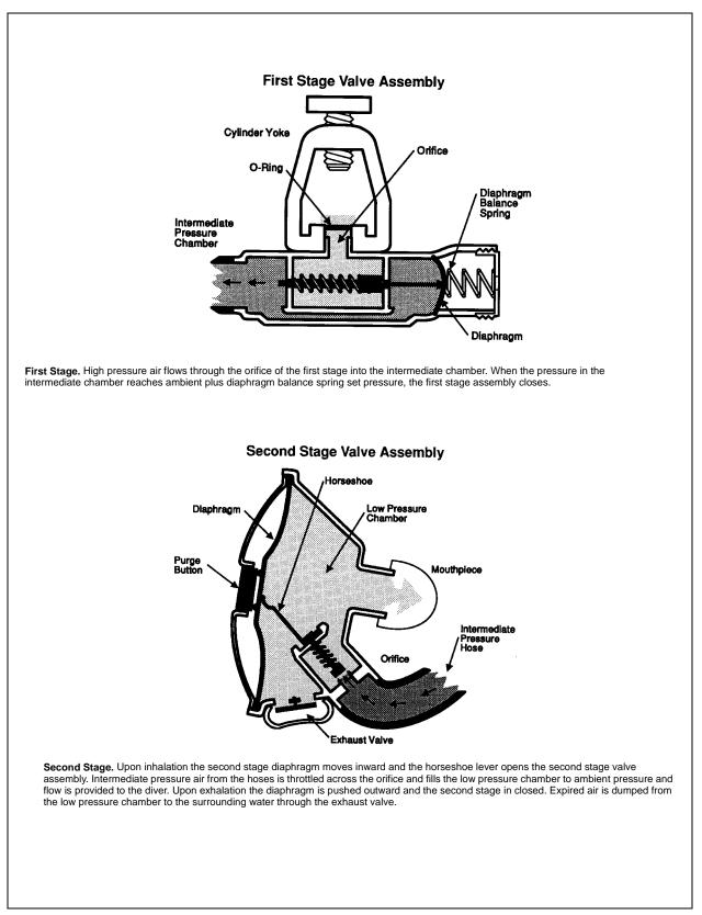
Figure 7-1. Schematic of Demand Regulator.
