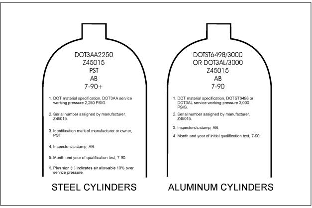
Figure 7-3. Typical Gas Cylinder Identification Markings.
